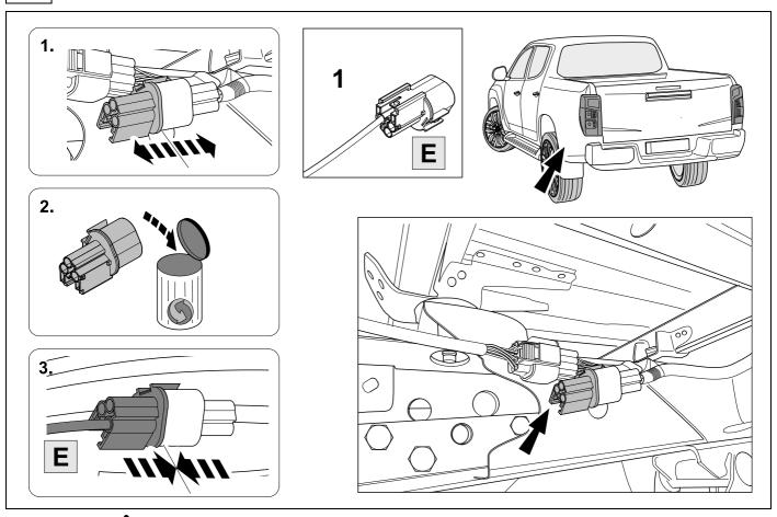
Module to be fitted out of the way on the chassis rail so that it is not submersed in water or exposed to direct dirt blast. Also ensure you use sufficient tie straps to secure the harness close to the module to minimize pulling on the module.
